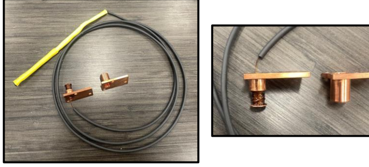
Figure 56: Magnet spindles Superconducting NbTi wire is spin around a copper spindle and two leads are fed out the top, which are then twisted and soldered to pins that mount to the dilution refrigerator’s DC drive lines. This magnet has long leads that breakout at the 4 K stage of the fridge, in a single piece, so that greater magnitude current can be drawn without heating the base stage of the fridge.
